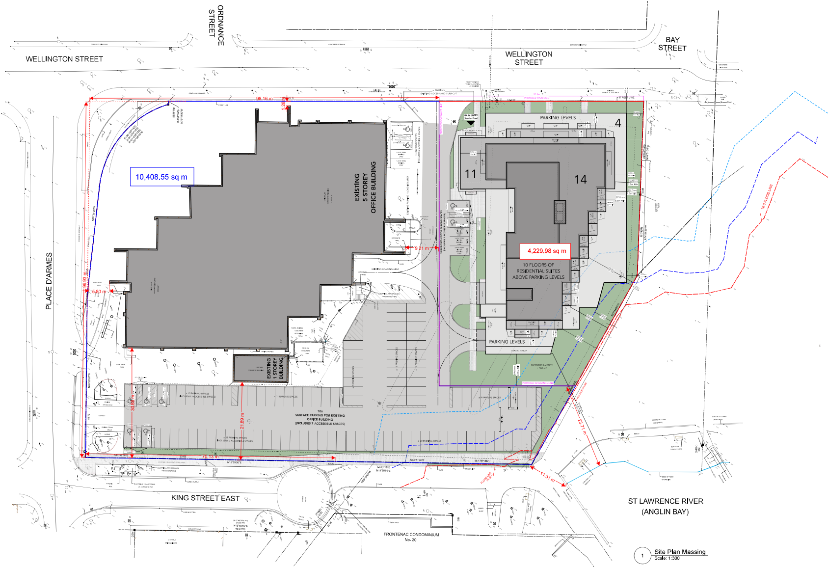
Appendix A - Arcadis markup of proposed site plan for future development at 279 Wellington Street
