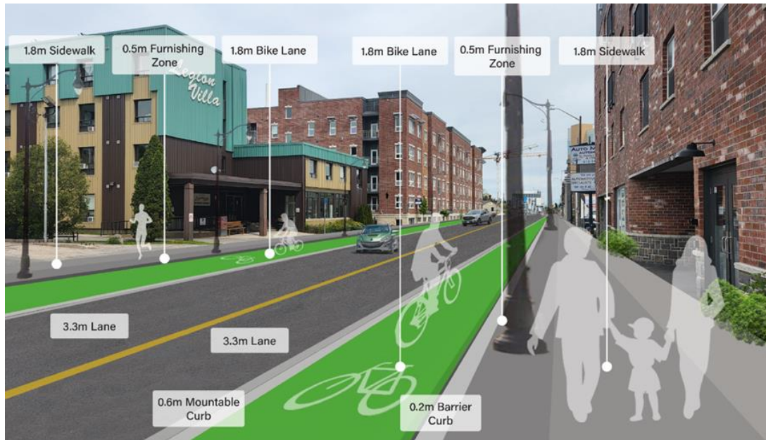
Figure 4: Adopted Willamsville Cross Section Road Modifications
