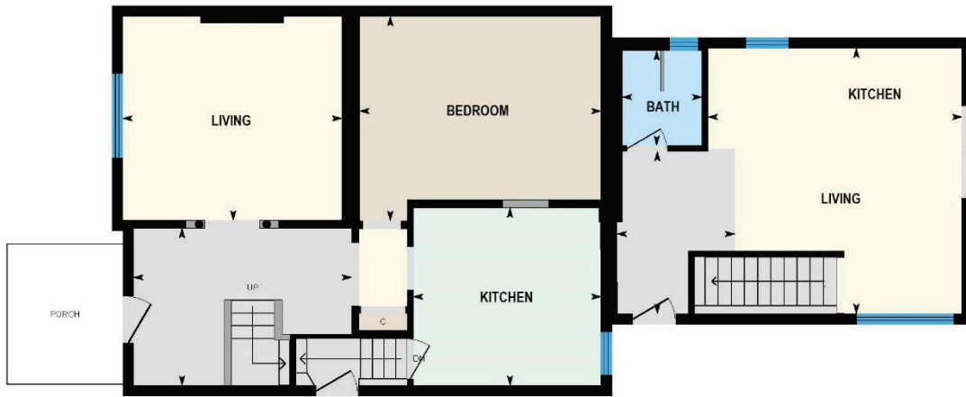
Figure 9 - Proposed Floor Plan - Main level
