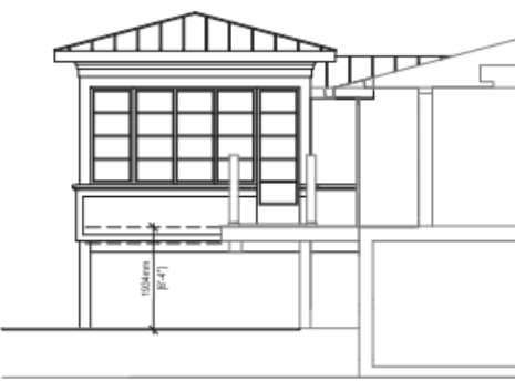
5 Proposed Elevation as viewed from Deck A03 1:100
