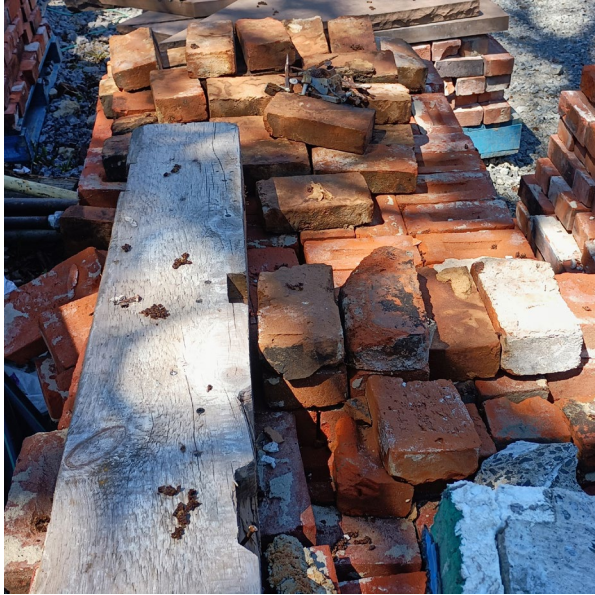
Figures 1 & 2: Dismantled bricks and replacement samples.
