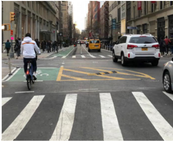
Enhanced Pavement Markings
