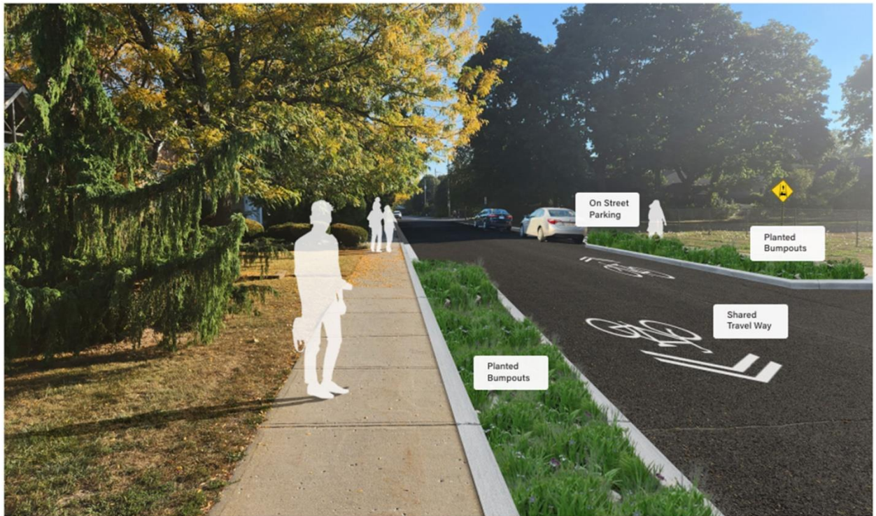
Figure 17: Typical 20 Metre Right-of-way Neighbourhood Bikeway
