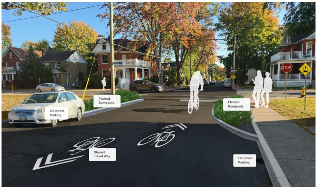
Figure 17: Typical 20 Metre Right-of-way Neighbourhood Bikeway
