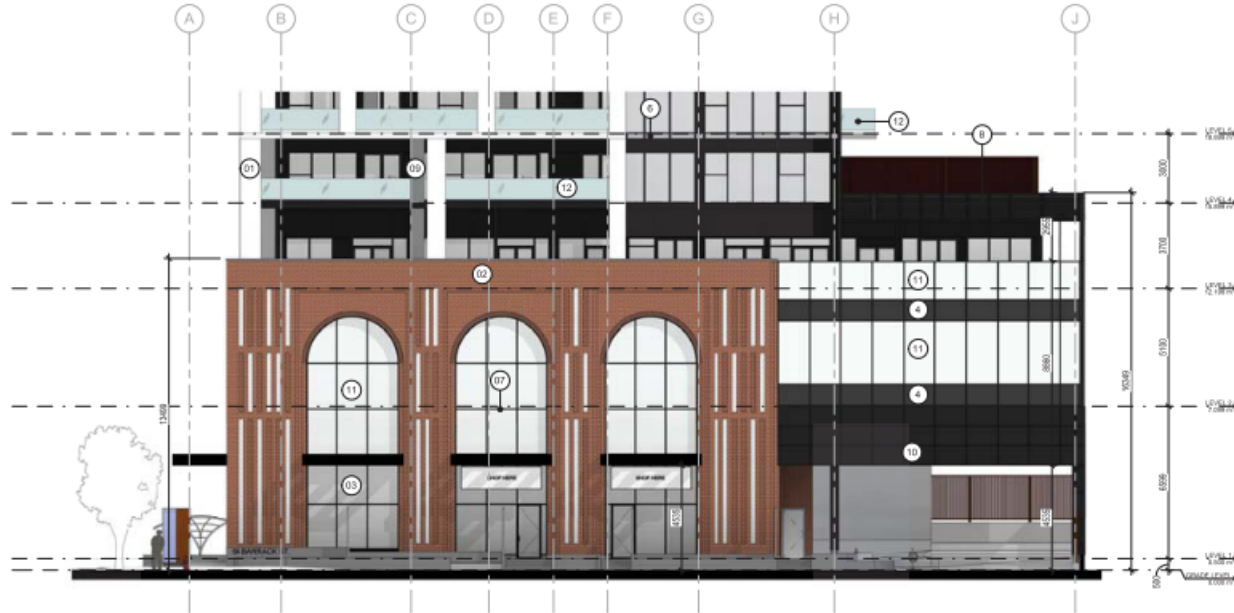
2 ENLARGED WEST ELEVATION - PODIUM WELLINGTON ST. 1:100
